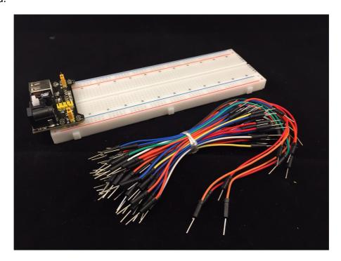
Our breadboard is a standard 64-holes one, capable of hosting few integrated circuits across the middle axis. The 'secret' of the breadboard is the 'direction' of the connections: The five holes between the middle line (where you put integrated circuits, normally) and the horizontal colored lines (blue and red, for negative and positive supply voltages) are connected VERTICALLY, while the power supply lines are connected HORIZONTALLY, from end to end.
